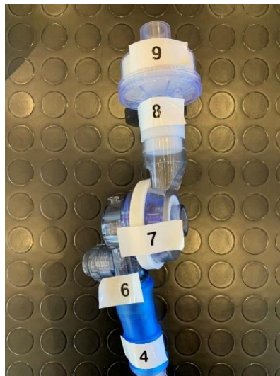
Figure 4.15: ABU PEEP valve group assembling part 2
