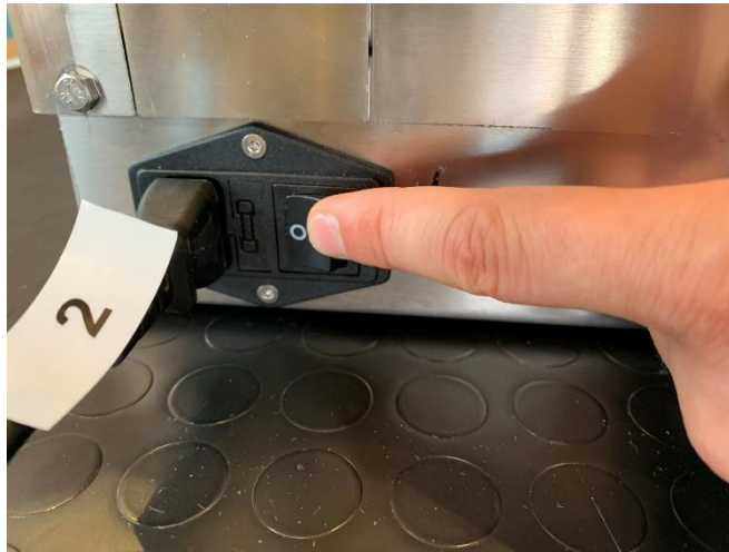
Figure 6.32. To turn off the ventilator, first set the I/O switch to the O position
