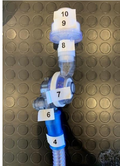
Figure 4.16: ABU PEEP valve group assembling part 3
