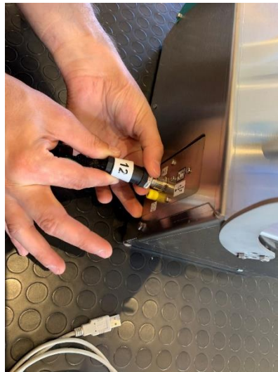
Figure 4.19: Connecting the ABU sensor pack cable to the ABU sensor pack cable port.
