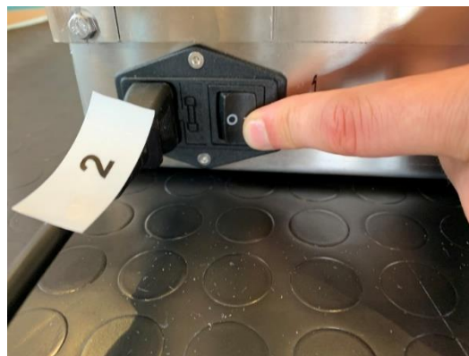
Figure 6.1. Turning ABU ventilator on using AC external (main) power supply.
