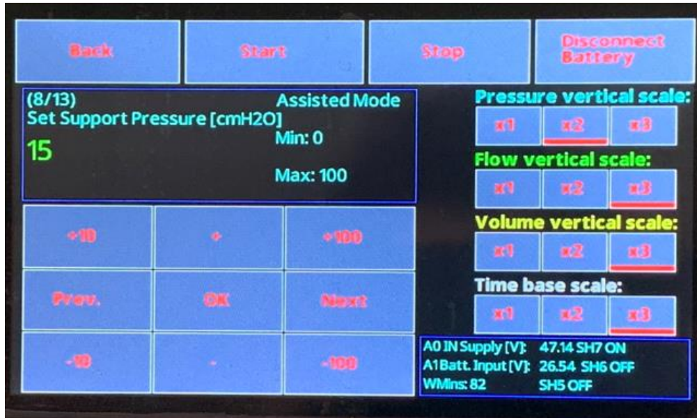
Figure 6.22. Setting Support Pressure
