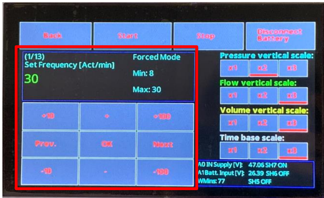
Figure 6.10. 'Setup' page panel to control ventilation parameters.
