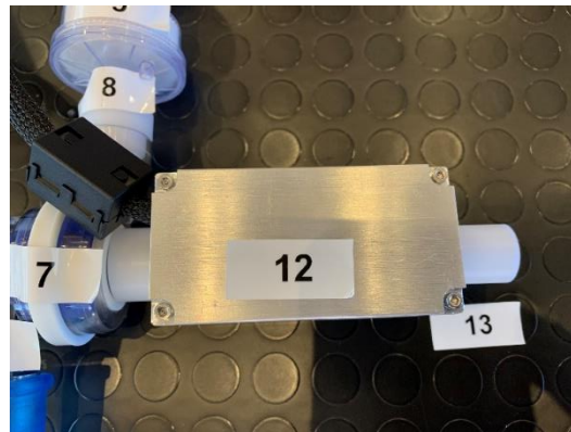
Figure 4.24: Connection of ABU sensor Y-connector fitting to the ABU Sensor Pack.
