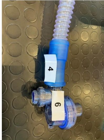
Figure 4.12: Connection of the ABU Check-valve to the breathing hose.
