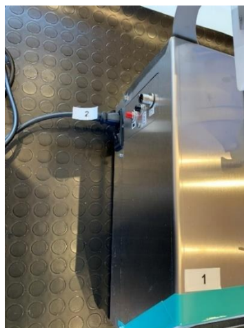
Figure 4.1. Connecting the AC power cable to the ventilator.
