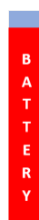
Figure C.4. Icon appearing on the left of the ‘Home’ page when the ventilator is functioning with its internal battery.
