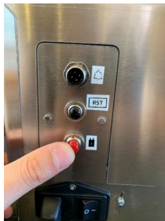
Figure 4.3. Press the Battery Start Button and hold it for more than 2 seconds to turn on the ventilator using its internal battery
