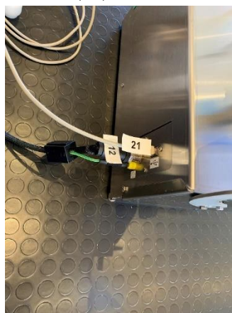
Figure 6.34. Connecting the ABU USB cable to the ABU USB port.
