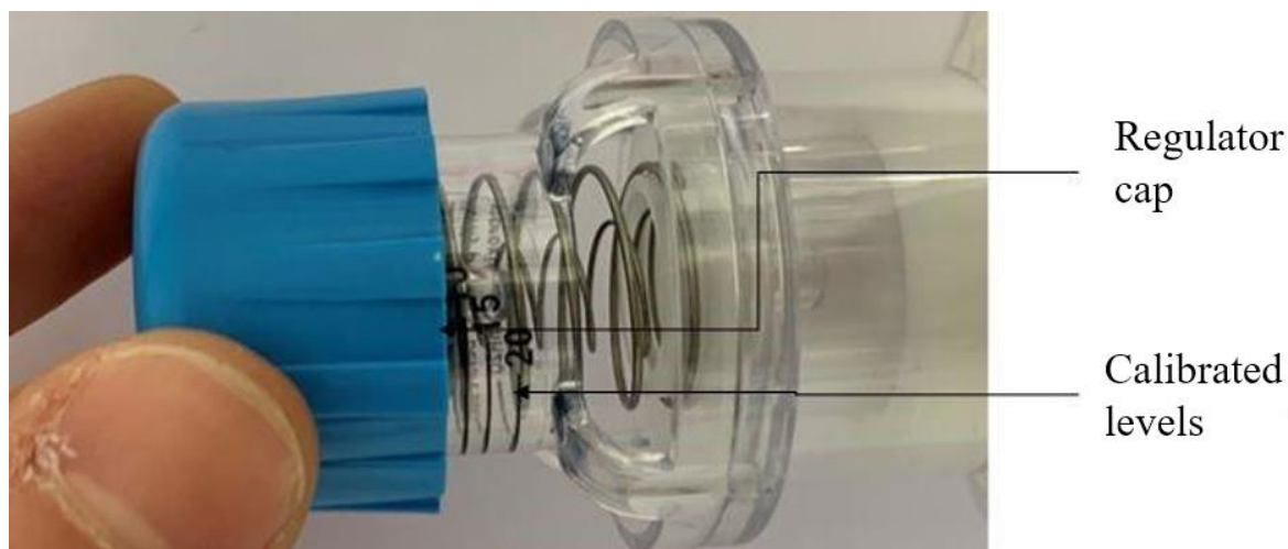
Figure 6.5: Adjustment of the PEEP valve.
