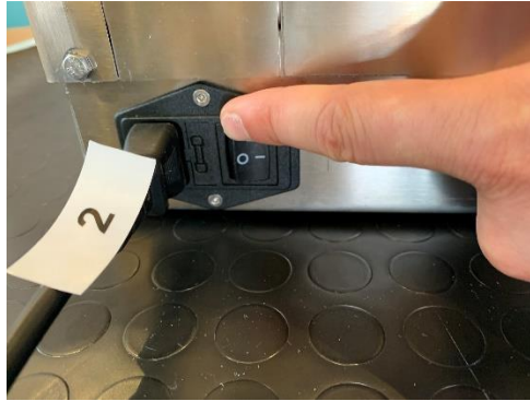
Figure 4.4. Set the I/O switch to I position in order to turn on the ventilator using the external AC power supply
