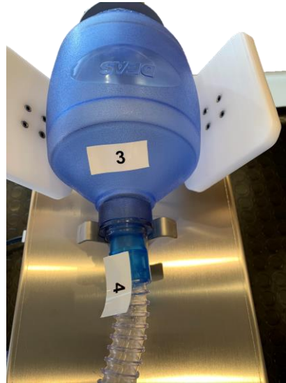
Figure 4.10: Breathing hose connection.
