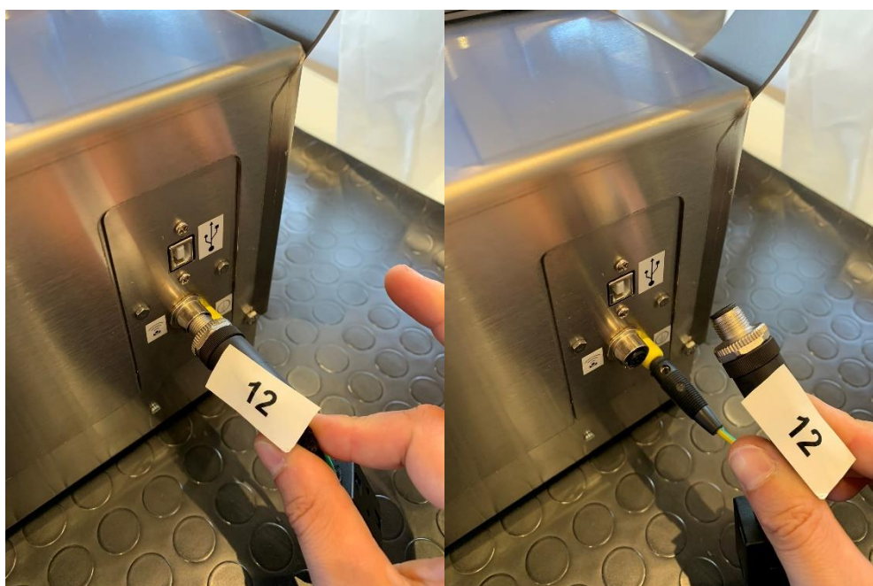
Figure C.1. ABU sensor pack test. At the beginning of the test the ABU sensor pack cable is connected to the ventilator (left); to perform the test the same cable must be disconnected as shown above (right).
