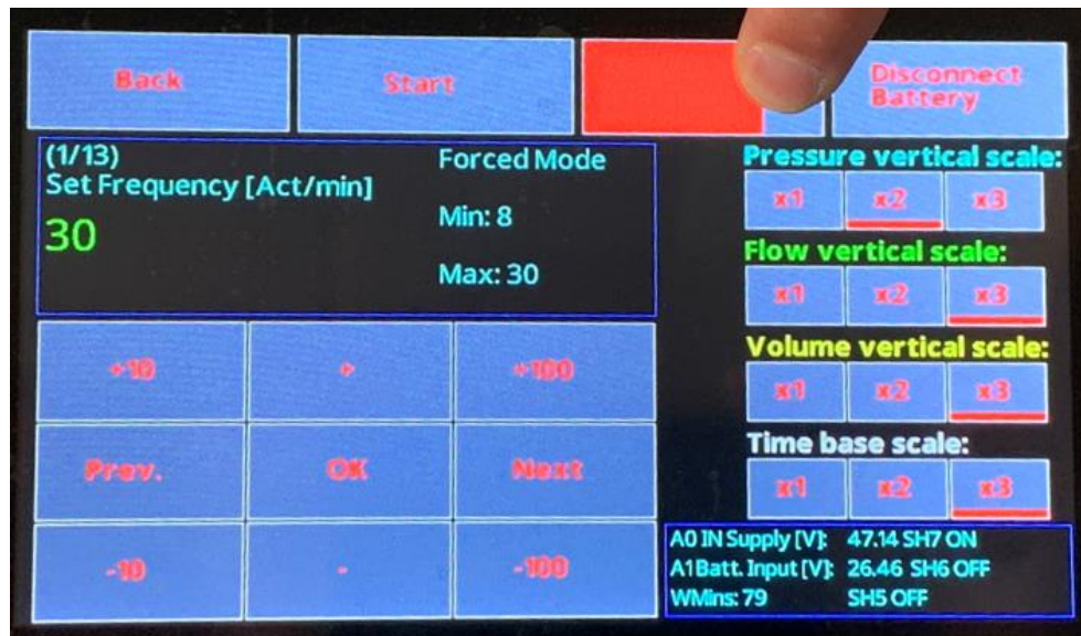
Figure 6.31. Stopping the ventilation. To stop the ventilation push and hold the ‘Stop’ button until the red bar completely covers the button as shown.
